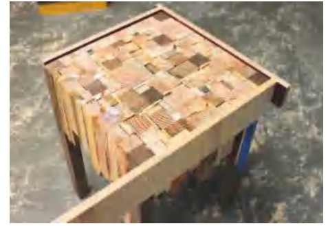
▲ Pic.5 Adding a level edge to the table top gives the router something to float on
